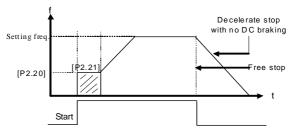
Fig6-1 Start and stop freq. output curve
