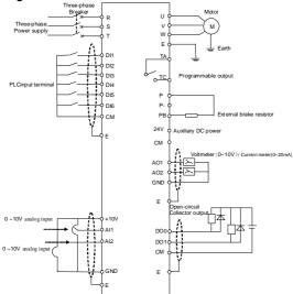
Fig.3-3 V600 series of inverter basic wiring
