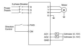
Fig9-1 Basic wiring
