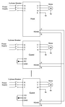
Fig9-4 Basic wiring
