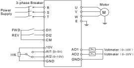
Fig9-2 Basic wiring
